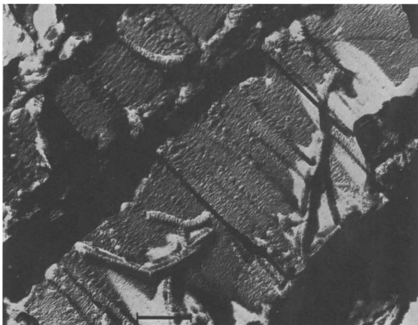
Figure 2 —Same as in Figure 1 but annealed at 120°C for one hour before fracturing
